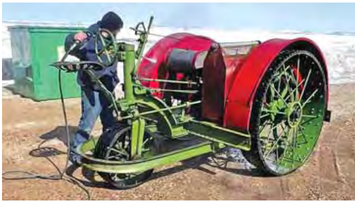
Ford Model B's most significant contribution to agriculture may be its faulty engineering. Complaints about it led to what became the Nebraska Tractor Test in 1920.
