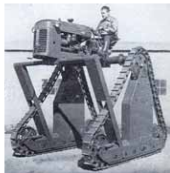
In the 1950s, this strange-looking triangular track tractor was used in California to spray sweet corn and detassel seed corn.
