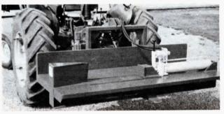
mel, is to hook a trailer on behind the tractor and splitter, go to the woods, cut and split a trailer-full, throwing into the trailer direct from the splitter table. Then, he says, you can return to headquarters with your chain saw and other tools carried on the splitter table.
