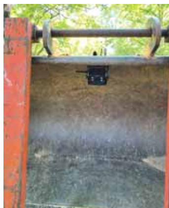
Magnetic mount attaches camera to bucket (left). Camera feed shows forks attached to the bucket (right).
