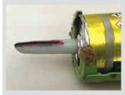
Cal Miner, Willmar, Minn.: "When using a caulking gun, you can lose track of where the angle cut is on a caulking tube. I put a black line on it to the point so when the tip gets messy, I just have to look at the line and I know what angle it's from.
