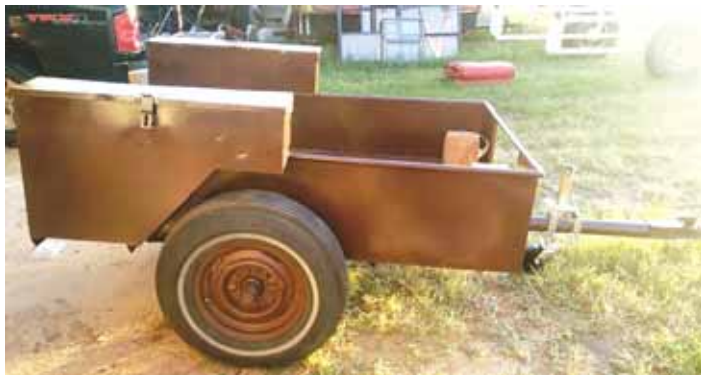
Surber built a custom trailer to haul his 1972 Miller Big 40 welder. It has angle-iron rails on the floor and two side cabinets for supplies.
