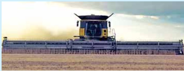
MacDon 61-ft. header center section moves up and down as the wings move up and down.
