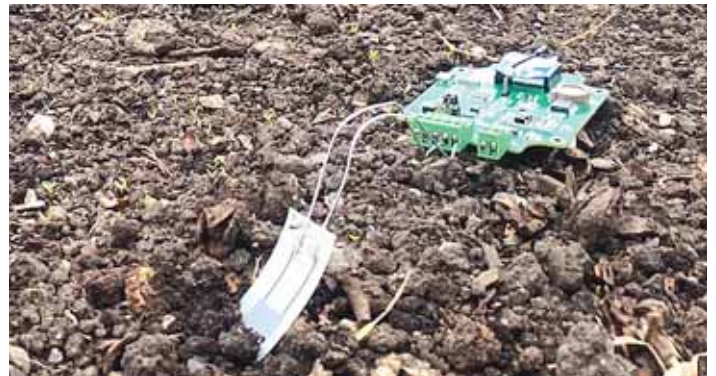
Biodegradable sensor (left) is partially submerged in the soil. Reusable electronics, which will help enable digital agriculture readings, are connected by wires.
