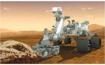
Laser creates a plasma of excited atoms and ions, which emit a light spectrum that the sensor can analyze. The multi-channel spectrometer measures thousands of data points.
