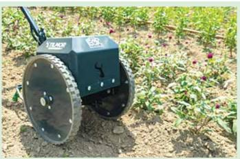
Electric hoe has a runtime of up to 70 min., and can cultivate, hoe, hill, mow, haul
