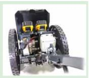
E-OX electric hoe has five speeds and can operate from 20V or 18V batteries from Dewalt, Makita or Milwaukee.
