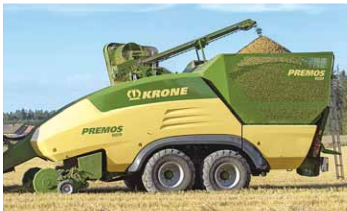
The Premos 5000 can be operated as a stationary machine. A foldable bale feeder with automatic twine removal for large square bales can be added.
