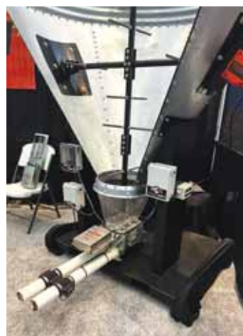
BridgRid's product is an internally mounted grid system that can be installed in nearly any sloped bulk container with a bottom discharge.
