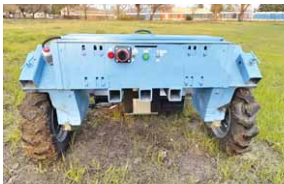
While the basic unit is intended for draft purposes, the 10 receiver hitches in various locations offer a wide range of options.
