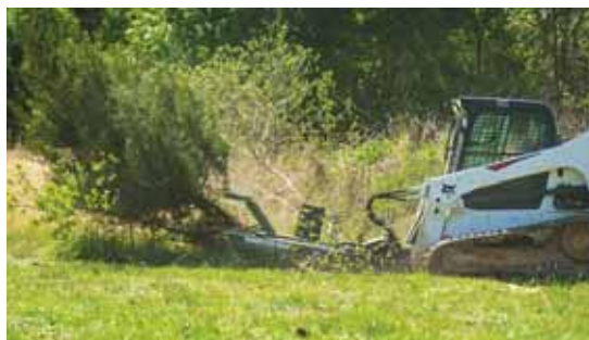
Reaper attachments are equipped with three 5/8-in. AR400, non-welded, bidirectional blades for quick and easy field change-out.
