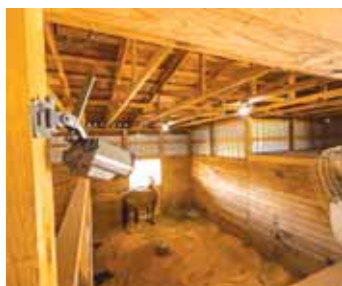
Motion-sensitive camera has its own battery and can be charged via an add-on solar panel.
