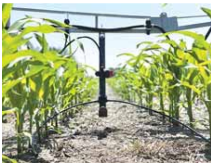
Drop lengths are 30 and 40 in., and a Dial-A-Rate feature allows farmers to change flow rates with a twist of the hand.
