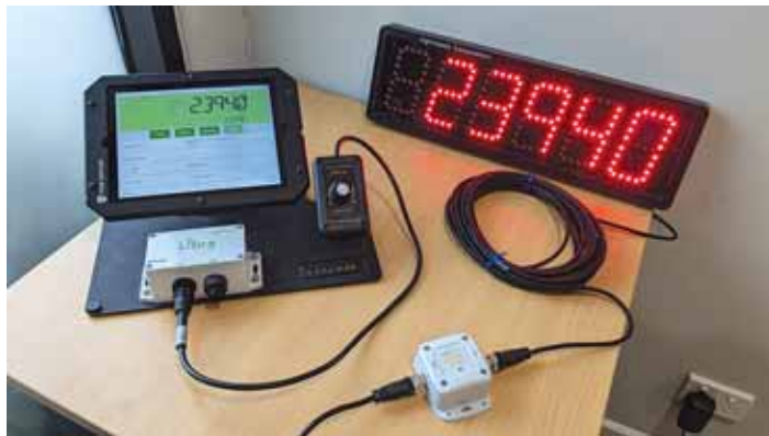
Agrimatics offers the addition of Serial Link, an external LED scoreboard display to view live grain cart weights from the Libra Harvest app.
