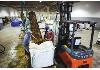
Kelp is loaded onto a conveyor that carries it to an IBC tote for fermentation.
