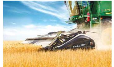
The Falcon achieves its fuel and time savings by utilizing cupped fingers that rotate at high speeds. They strip the heads of the crop and avoid processing the bulk of the crop residue.
