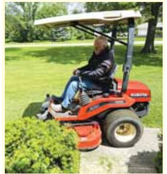
Roof from an old golf cart was bolted to the frame of ZTR, providing shade from the sun.
