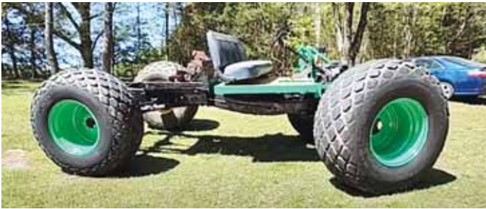
Floerkey repowered the big Ford with a 6 1/2-hp Predator 212 engine. He mounted the F350 hubs in the 26-in. wheels and rebuilt the clutch to mount a chain drive from the Predator driveshaft to the F350 drive.
