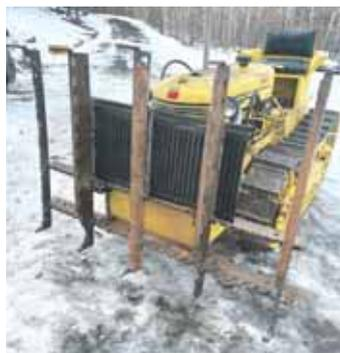
Vertical bars are pointed to pick up brush tight to the ground. Draw pins make changing back to the dozer blade quick and easy.
