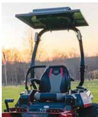
**CoolTops have a built-in 12-volt electric fan that runs from the tractor or mower battery.**
