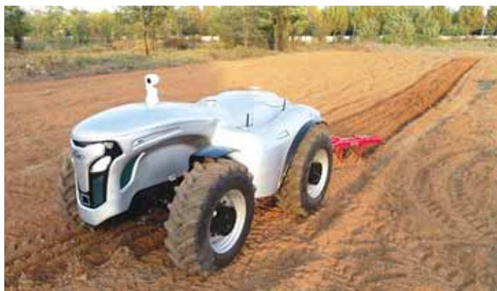
**YTO 220-hp. cabless tractor has an operating error rate of less than one inch.**
