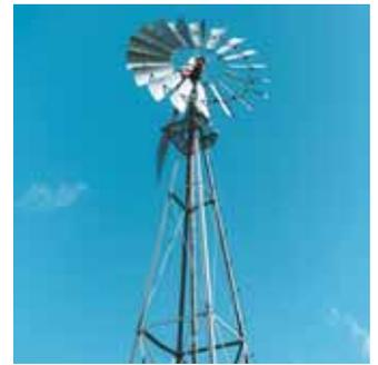
Windmill sizes range from 30 to 80 ft., with 6 to 16 ft. diameter wheels.
