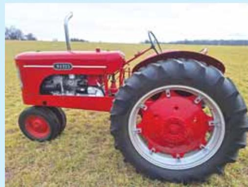
Built in 1952, it originally had a dual exhaust, 6-cylinder industrial engine with fluid drive Chrysler coupling and a New Process 5-speed transmission.
