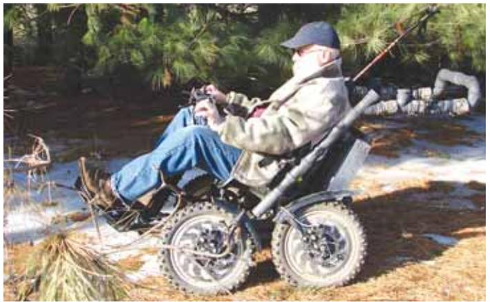
With two lithium batteries that fully charge in 4 to 6 hrs., running time is about 2 hrs. and 20 miles, depending on the terrain.
