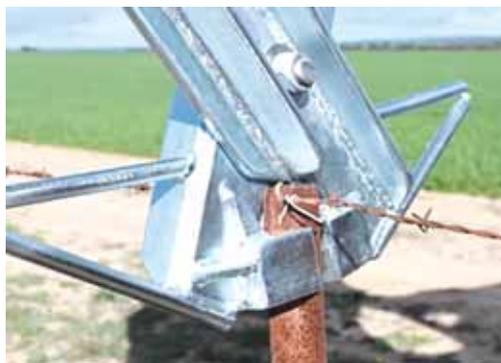
**Post-Pulla uses a scissors action to grip little more than the top inch of a post. Mounted to any type of front-end-loader, it grips the post tighter as upward force is exerted on it.**
