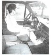
There's nothing on the market like this removable pedestal mount I made for our 1992 Ford pickup to hold the electric brake controls for a tow-behind trailer. It's extremely handy, right at your finger tips. We also liked not having to damage the dash of our new truck to mount the controls in the usual fashion. The stand could also be used to hold a cellular phone.
