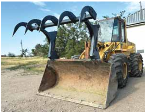
Justin Lutz designed and built a custom grapple fork for a 2 1/2-yd., heavy-duty bucket.
