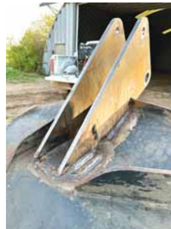
Mounting brackets for the grapple arms are 3/4-in. thick steel welded to the back of the bucket, reinforced with 1/2-in. plate steel.
