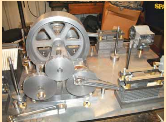
Partially completed view of engine shows detail all designed and cast by Dossdall.
