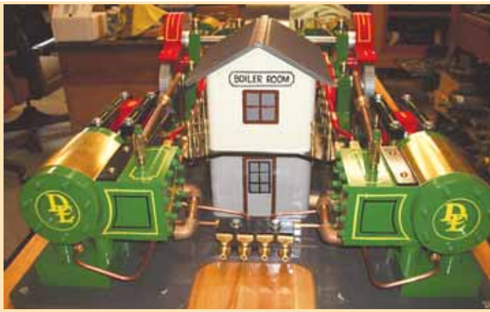
An overall view of Rich Dossdall's 4-cyl. engine shows intricate parts design, construction, and detailing. The exhaust stack and block housings are cast metal with milled grout lines.
