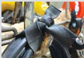
**Henry Lehman, Corvallis, Ore.:** Henry likes using strips of rubber inner tube to hold extension cords and hoses. "They're easy to tie, hold tightly, and they make it easy to hang stuff on the walls."
