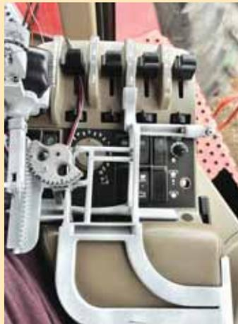
Armrest overlay with throttle control in RC tractor.
