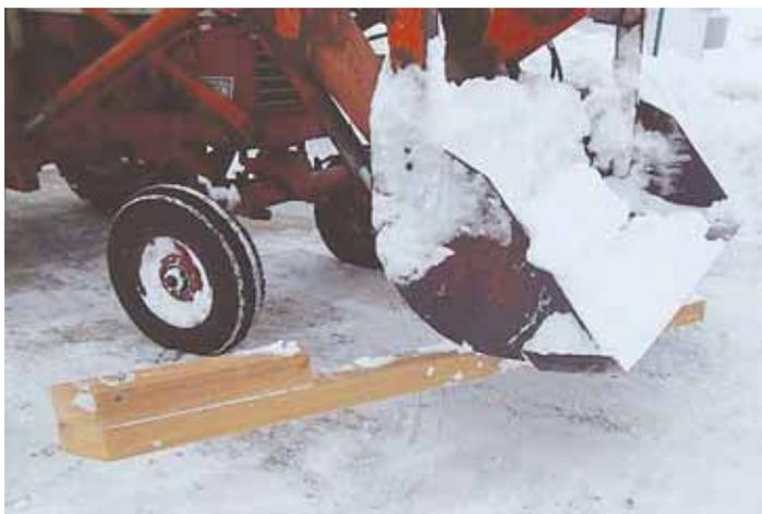
Beam extends out from the bucket’s right side about 4 ft. at about a 30-degree angle.
