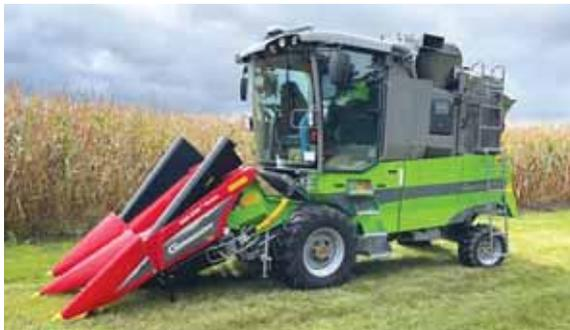
What makes the downsized combines so popular is they fit small-scale trial plots, typically around 15 ft. in length and 5 ft. in width.
