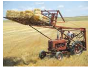
The Ranch Hand was a self-propelled version of an F-10 loader. This survivor was sold at a Montana auction in 2020.
