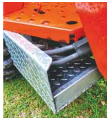
Lynn protected his tractor from future damage by fabricating a cover with diamond plate.
