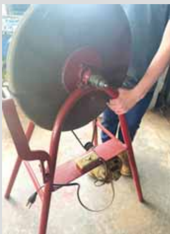
Shaft rides in two pillow-block bearings mounted to the pipe frame. A large diameter pulley mounted on one side of the shaft is bolted to one of the sandwiching plates.
