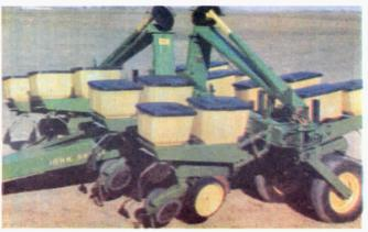
Kelderman's manually operated, fold-forward kit adapts to any rigid 5-in. or 7-in. toolbar.
