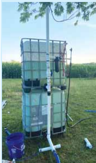
Wood placed two 270-gal. IBC totes, one on top of the other, on the highest point of his farm for a water tower.
