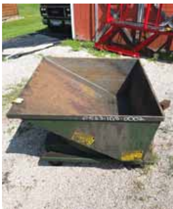
Half yard 4,000-lb. dump trailer made from an industrial dump hopper.
