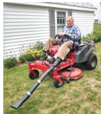
Baughn uses the blower's 6-in. flat nozzle and extra tubes to reach well ahead of the mower, about 4 in. off the ground.
