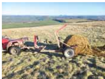
UK farmers built a bale unroller that can handle a full bale and be moved using an ATV/UTV.
