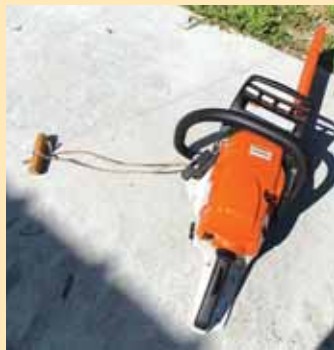
Starter rope extension made from clothesline with a wooden handle on the end helps to start saw while standing.
