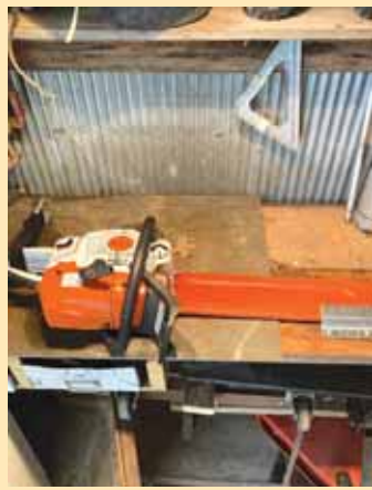
Metal bracket over blade holds saw in place with a bungee cord in the handle.
