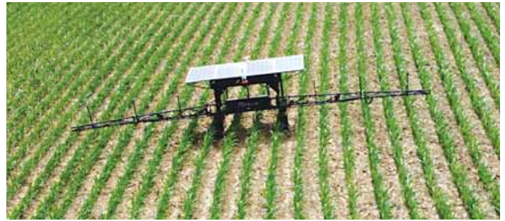
Robotic spot sprayer is powered by four solar panels and can spray up to 500 acres per day, reducing chemical use and spray drift.
