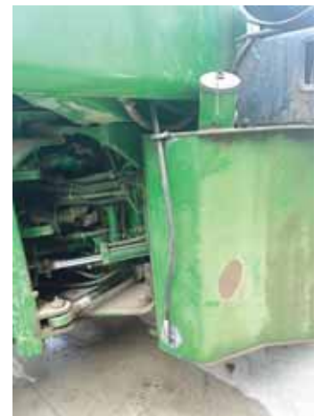
Wayne Hopper and his neighbor Bill Garniss fixed the fuel draw on a Deere 8650 fuel tank by installing a fitting 2 in. above the tank's bottom and running an outside line to the filters.
