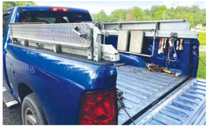
Sowinski made rugged side extensions for his pickup box out of used diamond plate running boards.
