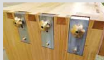
Planing stops on the toolbox are made of stainless-steel flat bar welded into an L-shape.
