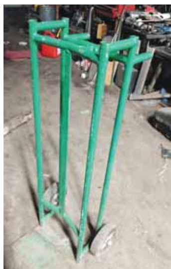
Bowen's handcart has a two-part frame that allows the wheels and frame to be folded in, allowing for side-to-side movement on the wheels.
