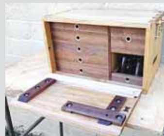
Chest opens to reveal drawers that store the various tools Dr. Al needs for box-making. Drawers are made with half-lap dovetails and brass pull rings.
