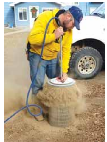
The rotating nozzle has three ports and a quick-connect mechanism to hold interchangeable arms. The arms are cut to size and kept 1 to 1 1/2 in. away from the inside of the radial sealed air filter.
