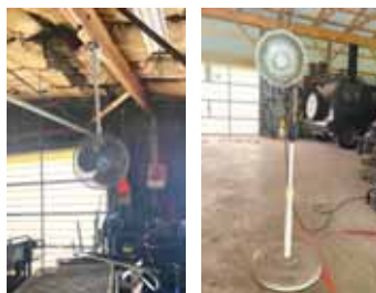
Fan mounted upside down to save space and fan mount used for shop light.
