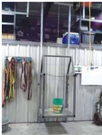
"I use the elevator to move heavier items to the overhead storage area in my shop, items that would be awkward to carry up the stairs," says Boyce.
