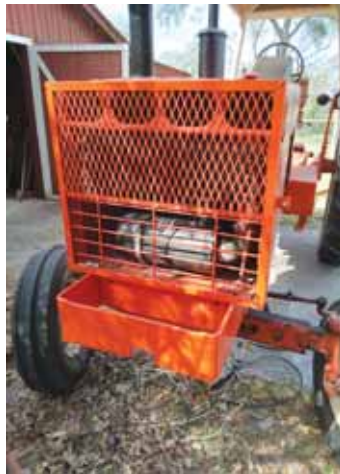
Barlow made his own grill for his AC 185 using scrap from around his shop.
