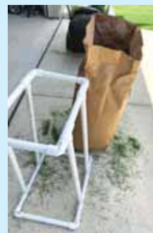
PVC frame holds yard waste bags for easy loading.
