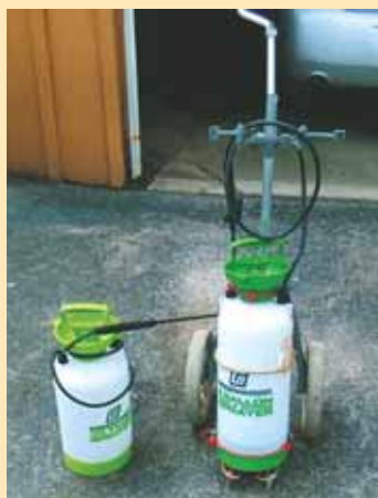
Golf push cart modified to carry a 2-gal. sprayer.
