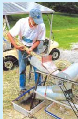
Howe's thresher has quick-change curved screens, variable pulley ratios, and a degree of inclination, allowing infinite setups to handle any processing.
