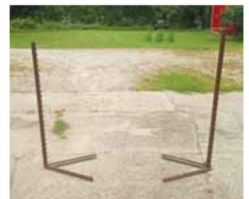
**Schantz trims posts to 4 to 5 ft. for the uprights. He cuts others into 18 to 20-in. pieces to use as bases. He welds two to each upright with a spread of about 18 in. at their farthest points.**
