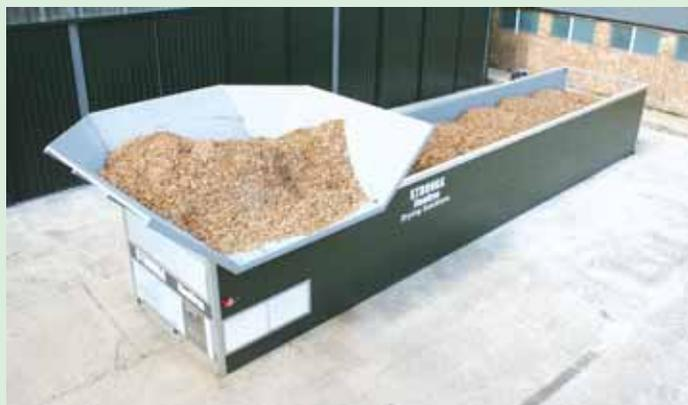
Top removed, showing hopper and drying beds.
