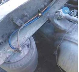
"Just cut the airline and plug in the DOT-approved fitting that reads the pressure on the air suspension," Riegel says. "Once calibrated, load whatever you're hauling and weigh on a certified scale, then enter those numbers into the application."
