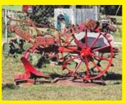
I have a self-propelled steel wheel 1-bottom plow made by Shaw. It has an early Briggs engine on it with a cast iron cover on the side of the belt and the lifting mechanism of the plow.
