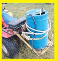
I built a carrier for a 50-gal. drum that connects to the trailer ball on my ATV. It's a salvaged folding tractor seat support. I mounted an old 1 7/8-in. ball hitch to it and ran 3/4 by 1-in. angle irons from the rear corners of the carrier to the rear rack on the ATV.
