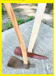
I found an adze head and put a straight handle on it. The cutting edge isn't sharp and doesn't appear to have ever been sharp. It has "US PAT D256322" on the underside of the blade. It looks very different from a conventional adze due to its long and heavy triangular point on the back of the head.
