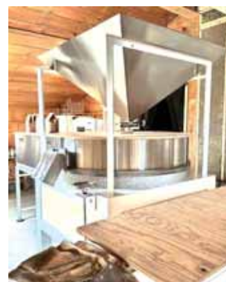
40-in. New American granite stone mill was installed in May 2023 and is capable of milling 100 lbs. of flour an hour.
