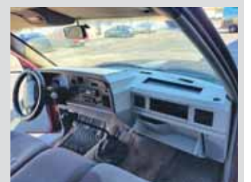
Designed to replace stock plastic dashboards, the piece weighs approximately 18 lbs. Customers can request custom setups based on the gauges or digital dashboards they want displayed.
