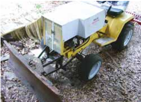
Rawls used a Harbor Freight 6-hp. engine and IH 404 clutch to rebuild his Cub Cadet.
