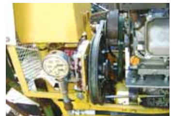
Hydraulic pump and drive pulley with centrifugal clutch and belt drive to driveshaft.
