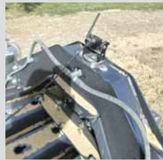
Remote camera can be mounted to show if equipment is working properly.
