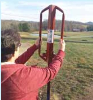
Redesigned Hammer Head spring recoil post driver lifts up on a recoil so users can concentrate on pulling it down.
