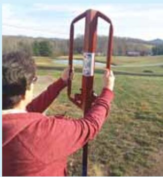
Redesigned Hammer Head spring recoil post driver lifts up on a recoil so users can concentrate on pulling it down.
