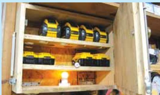
**Plywood box uses a low-voltage lightbulb to keep tool batteries from freezing.**
