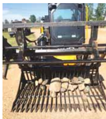
Imhoff converted a beach cleaner into a rock picker.
