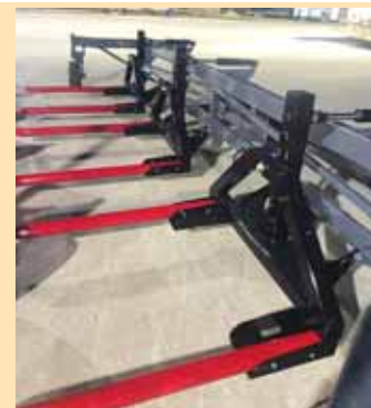
Pipes can move on the bracket to handle 4, 5 or 6-ft. bales.
