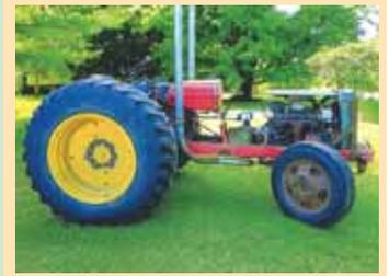
**Lilly used the frame, wheels, operator station, and drive train of a Massey 44 tractor coupled with a 350 V-8 Chevy truck engine.**
